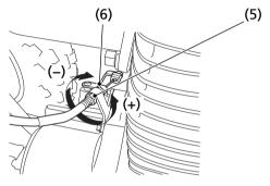
(5) lower adjusting nut(6) lower lock nut
