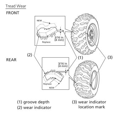
To check the condition of a tire tread, measure the groove depth (1) in the center of the tire, or check the wear indicator (2). For best performance, you should replace a tire before the tread depth at the center reaches the following limits:
