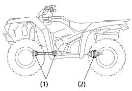
(1) propeller shaft boots(2) yoke joint boot
