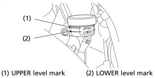
With the ATV on a level surface, check the fluid level. It should be between the UPPER (1) and LOWER (2) level marks. If the level is at or below the LOWER level mark, check the brake pads for wear (page 167).
