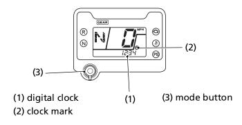
After the battery is reconnected (page 189), check the clock. Readjust the clock if necessary.
