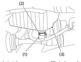
(1) drain tube(3) air cleaner housing(2) clip
