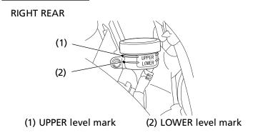
With the ATV on a level surface, check the fluid level. It should be between the UPPER (1) and LOWER (2) level marks. If the level is at or below the LOWER level mark, check the brake pads for wear (page 170).
