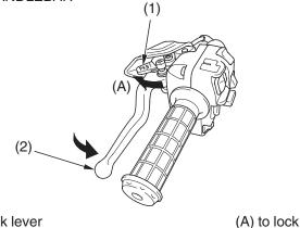
(1) lock lever(2) rear brake lever/parking brake lever
