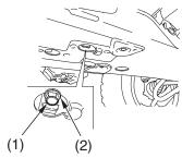
(1) engine oil drain bolt
