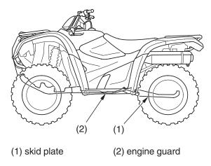
The skid plate (1) protects the rear final gear case.
