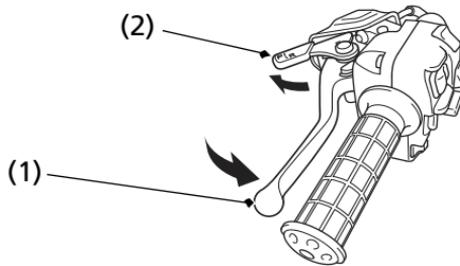
(1) rear brake lever/parking brake lever
