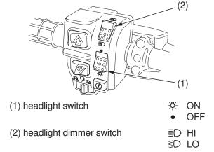
The headlight switch (1) is used to turn the headlight ON (  $\clubsuit$ ) or OFF ( • ). To operate, turn the switch to ON (  $\And$ ) or OFF ( • ).
