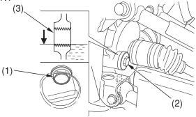
(1) oil drain plug(2) oil fill cap
