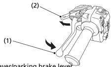
(1) rear brake lever/parking brake lever
