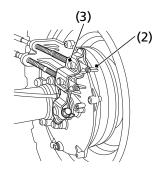
(2) brake lever adjusting nut
