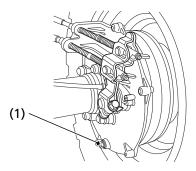
(1) rear brake drain bolt
