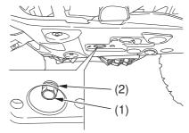
(1) engine oil drain bolt
