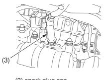
(3) spark plug cap(4) center electrode
