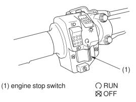
The engine stop switch (1) is used to stop the engine in an emergency. To operate, slide the switch to the OFF ( \bigotimes ) position. The switch must be in the RUN ( () ) position to start the engine, and it should normally remain in the RUN ( $\bigcirc$ ) position even when the engine is OFF.
