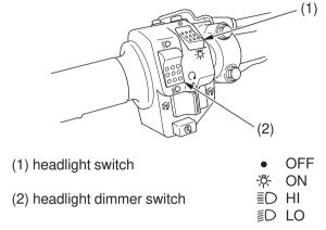
The headlight switch (1) is used to turn the headlight ON (  $\Rightarrow$  ) or OFF ( • ). To operate, turn the switch to ON (  $\Rightarrow$  ) or OFF ( • ).
