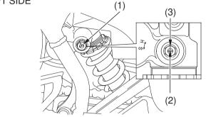
(1) compression damping adjuster(3) reference punch mark(2) punch mark
