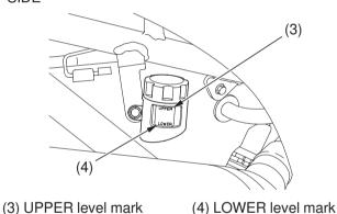
With the ATV in an upright position, check the fluid level. It should be between the UPPER (3) and LOWER (4) level mark. If the level is at or below the LOWER level mark, check the brake pads for wear (page 133).
