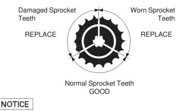
Use of a new chain with worn sprockets will cause rapid chain wear.
