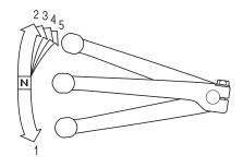
The shift lever is located near the left footpeg. One full stroke of the shift lever shifts the transmission to the next higher or lower gear in the shifting sequence. The shift lever automatically returns to the horizontal position when released.
