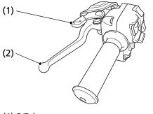
(1) P/R lever(2) rear brake lever/parking brake lever
