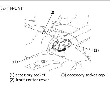
The accessory socket (1) is attached to the left side of the front center cover (2). You can use the accessory socket to power a trouble light, spotlight, CB radio, or cell phone, etc.
