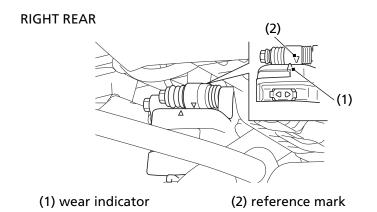
Check the wear indicator (1). If the wear indicator aligns with the reference mark (2), both pads must be replaced, see your dealer for this replacement.
