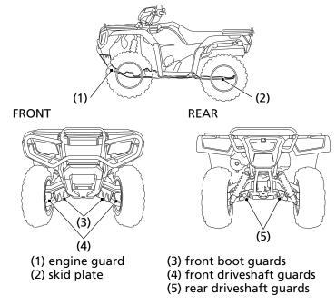
The engine guard (1) protects the engine crankcase.
