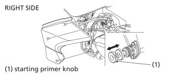
The starting primer knob (1) is located on the carburetor float bowl. The knob may be used when starting the engine in extremely cold weather ( $-15^{\circ}$ C,  $5^{\circ}$ F). See *Starting Procedure*, page 71.
