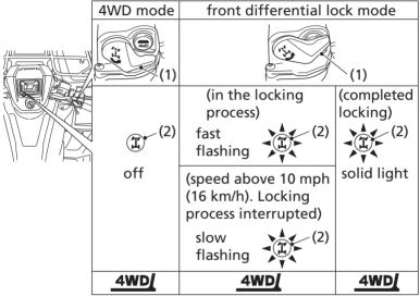
(1) differential lock switch (2) differential lock indicator
