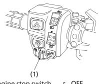
(1) engine stop switch r OFF e RUN
