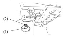
(1) engine oil drain bolt
