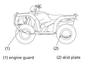
The engine guard (1) protects the frame, front final gear case and engine crankcase.
