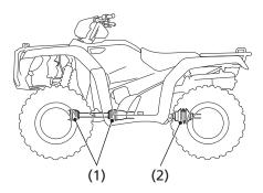
(1) propeller shaft boots(2) yoke joint boot
