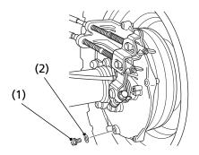
(1) rear brake drain bolt (2) sealing washer
