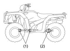
(1) propeller shaft boots(2) yoke joint boot
