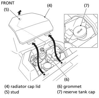
6. After adding coolant, reinstall the reserve tank cap.7. Install the radiator cap lid.
