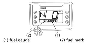
Regardless of what mode the display is in, when the fuel level reaches 1st segment (3), the display will automatically switch to the fuel gauge display. You should refuel as soon as possible.
