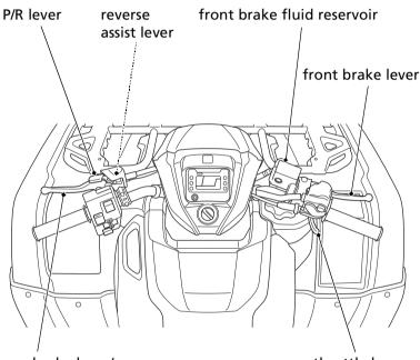
rear brake lever/ parking brake lever
