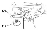
(1) engine oil drain bolt
