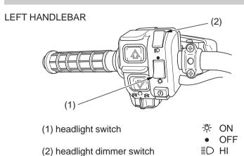
The headlight switch (1) is used to turn the headlight ON (  $\mbox{\ensuremath{\mbox{$\mbox{$\mbox{$\mbox{$\mbox{$\mbox{$}}$}}$}}$ ) or OFF (  $\mbox{\ensuremath{\mbox{$\mbox{$\mbox{$\mbox{$\mbox{$}$}}$}}$ ). To operate, turn the switch to ON (  $\mbox{\ensuremath{\mbox{$\mbox{$\mbox{$\mbox{$\mbox{$}$}}$}}}$ ) or OFF (  $\mbox{\ensuremath{\mbox{$\mbox{$\mbox{$}$}$}}}$ ).
