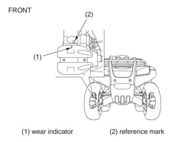
Check the wear indicator (1). Remove the front wheels (page 191). If the wear indicator aligns with the reference mark (2), both pads must be replaced, see your Honda dealer for this replacement.
