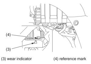
Check the wear indicator. If the wear indicator (3) aligns with the reference mark (4), replace both pads as a set, see your Honda dealer for this service.
