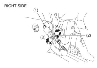
(1) rear brakelight switch(2) adjusting nut
