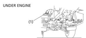
(1) engine oil drain bolt
