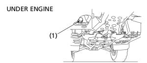
(1) engine oil drain bolt
