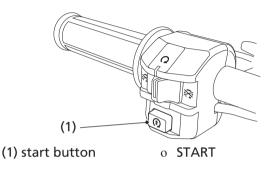
The start button (1) is used for starting the engine. Pushing the button in starts the engine. See *Starting Procedure*, page 56.
