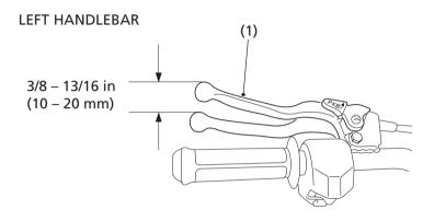
(1) rear brake lever/parking brake lever
