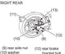
(10) washer bracket bolt (11) protective tape (13) rear brake bracket
