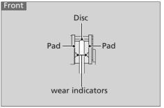
**Front** Inspect the brake pads from the bottom of the brake caliper.
